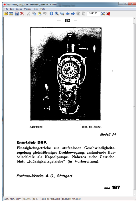
Figure B12 - ScanTailor colour mode setting: Black and White Quality of the photograph is very bad, Output file size of TIFF-ZIP is 48KB. Do not use this setting for such types of sources!
